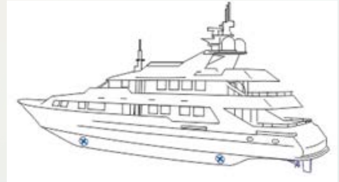
BTT + STT + Rudder + CPP
